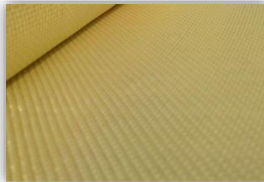
Figure I-9: Fibre d'aramide [10]
