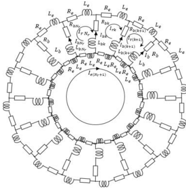
Figure 3.2: The equivalent circuit of the rotor squirrel cage (Shi et al,2013).
