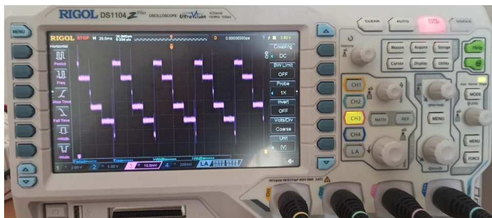
Figure IV- 18 : The cost function signal for MPC controller.
