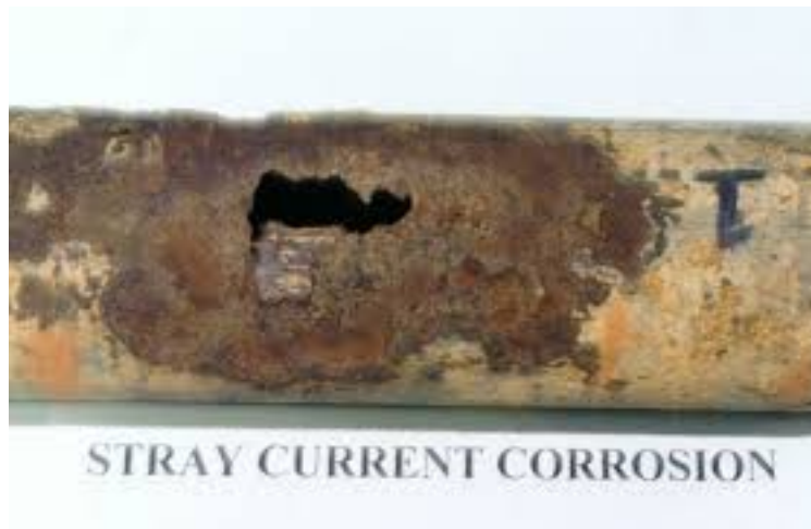
Figure 4.2: Stray current corrosion.
