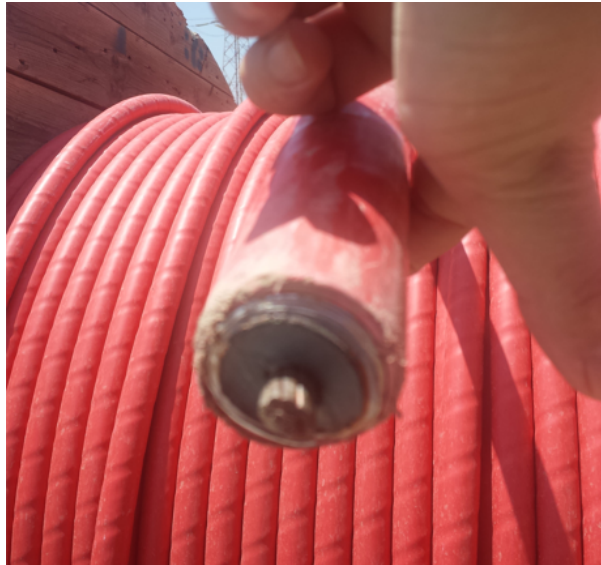
Figure 2.6: High voltage(30KV) cable
