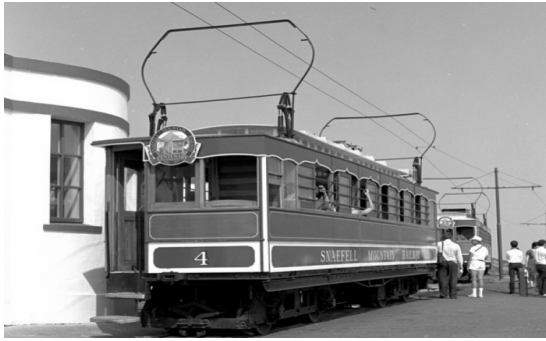
Figure 1.8: Bow collector system.
