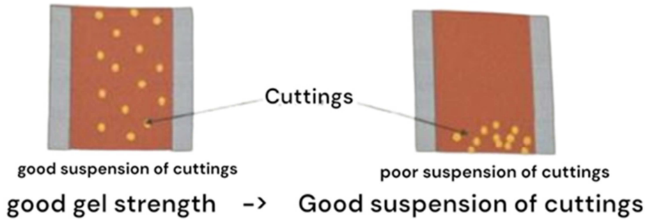
Figure 13 - The gelling power of the drilling fluid
