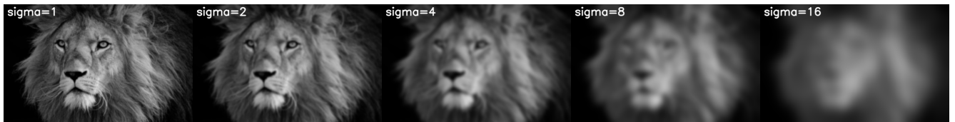
Figure 2.4: Gaussian scale-space filtering: results with sigma values from 1 to 16
