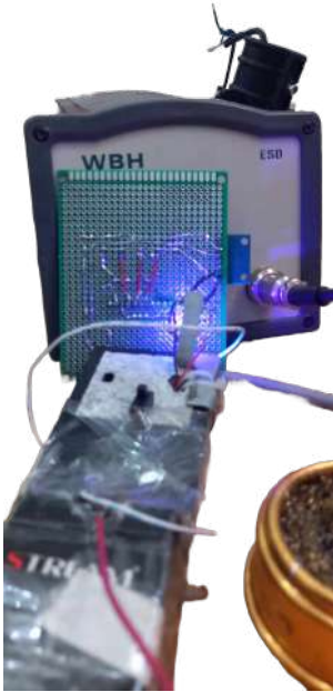
Figure 3.10: UV Exposure After Applying Solder Mask
