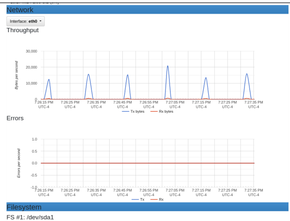
Figure 4.9: Network Throughput and Errors Monitoring with cAdvisor for the Web App
