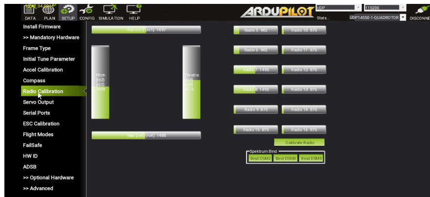
Figure 3.10: Visualization of PWM signals on Mission Planner
