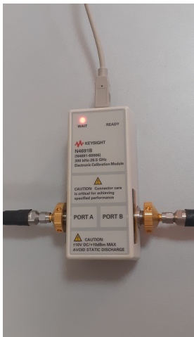
Fig. 15: Calibration kit in OFF state.
