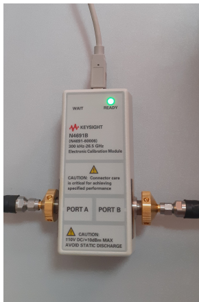
Fig. 16: Calibration kit in ON state.
