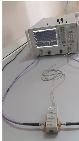
Fig. 15: Calibration kit in OFF state.
