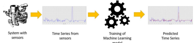
Figure 8: Process of condition monitoring [3].
