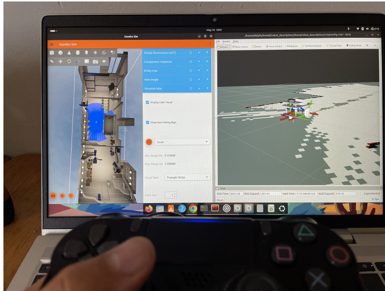
Figure 5.9: SLAM-based mapping using joystick in a Gazebo environment.
