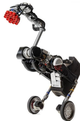
Figure 2: Example of a hybrid mobile robot: a wheel-legged robot with an articulated arm.
