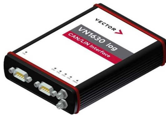
Fig.2.5.The VN1630 CAN Case by Vector Informatik
