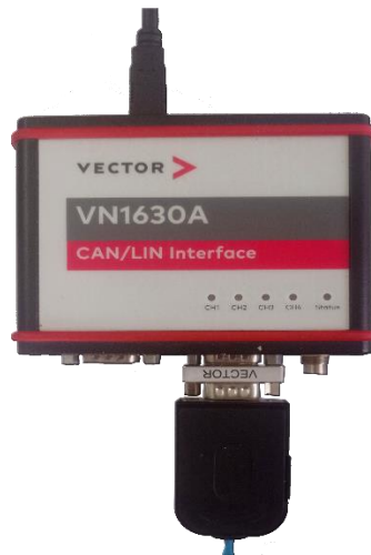
Fig.2.8. A picture of a DB-9 connector connected to VN1630 CAN Case
