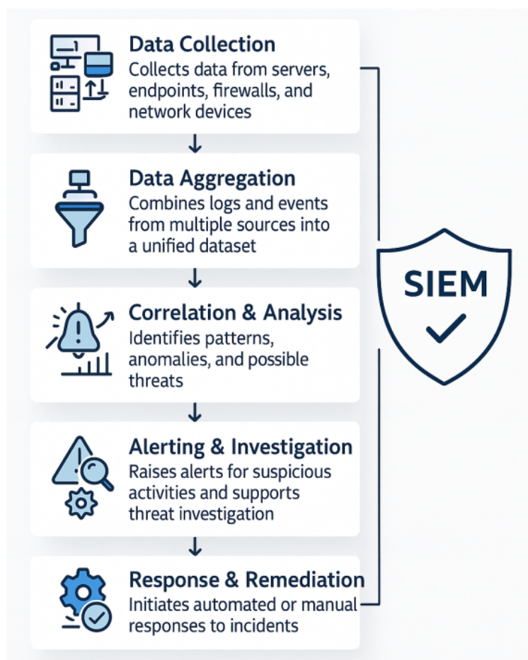
Figure 1.3: SIEM Functional Process
