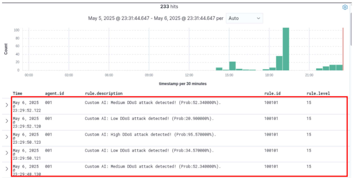
Figure 4.16: DDoS Attacks Alerts by The CNN-LSTM Model on The Wazuh Dashboard (File Based Integration Method).
