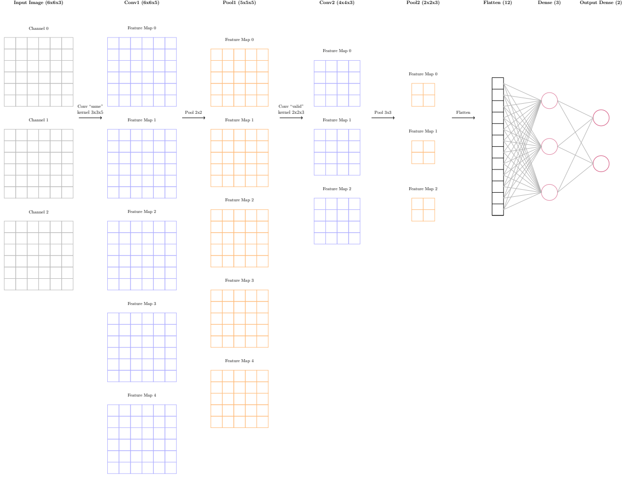
Figure 3.3: Simple example of a CNN architecture
