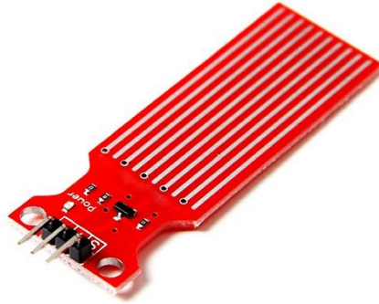
Figure 3.6: Rain Drops level sensor
