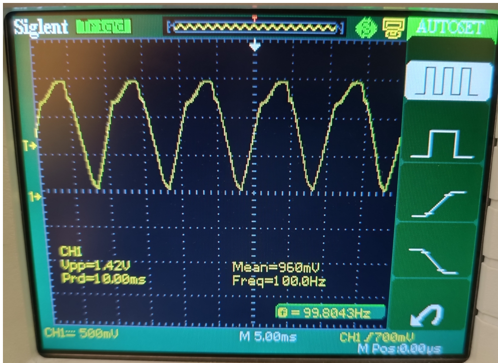
Figure 45. Rectifier Output Voltage.
