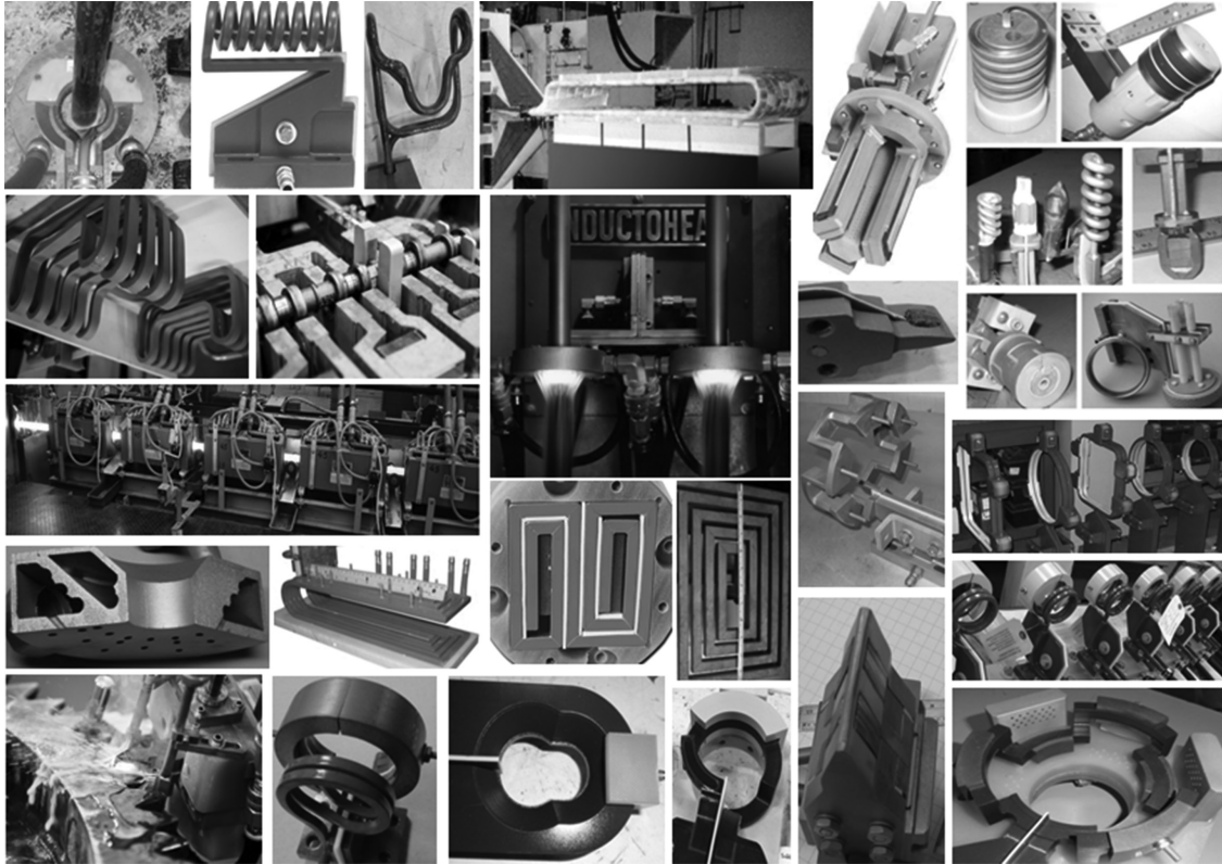
Figure 1. A variety of geometries of heating inductors used in IH systems.[1]
